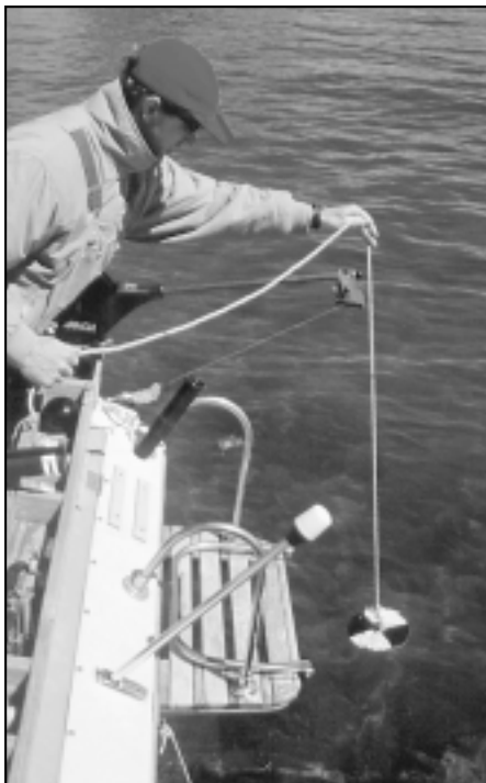
A CSLAP volunteer measures the water clarity by lowering a Secchi Disk into the water until it is no longer visible.
