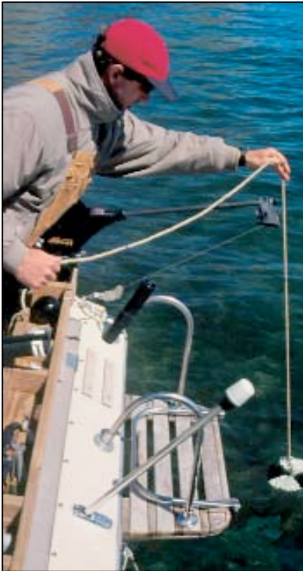
To measure water transparency a black and white Secchi disk is lowered into the lake until it is no longer visible.
